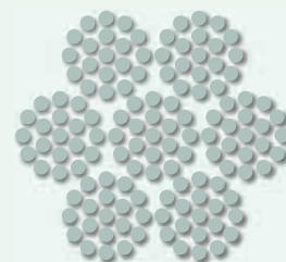
↑ Inox-Seil WC Câble Inox WC Stainless steel wire rope WC 6 x 19 + WC E = 1,0 – 1,3 · 10 5 N/mm 2
