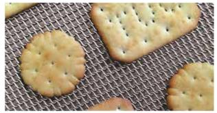
Compared with solid steel or multiple spiral belts our rolled baking oven belts allow gases in the product to escape also downward during the baking process, so that no unwanted bubbles will appear at the reverse side of the product. Moreover, the bottom side shows an appealing characteristic pattern.
