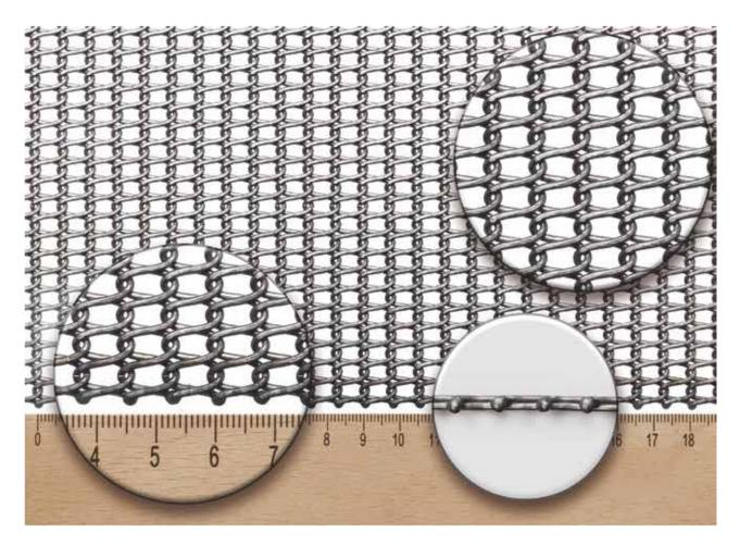
Rolled baking oven belts, also known as Z-Belts, are made of round wire spirals with very narrow and equal tolerances. The coiling direction of the spiral is changed with each wire, while they are intermeshed in pairs into each other (i.e. "double weaving"). The wire fabric is rolled flat first with greatest care before the belt is cut to width and the edges are spot welded. With this a very smooth, equal and angular belt structure is achieved with
